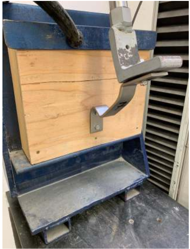
Figure 6b. Typical failure mode.
