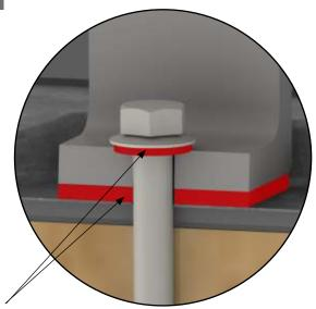
EPDM sealing washer and K2 EverSeal gasket on L-Foot ensure watertight seal.
