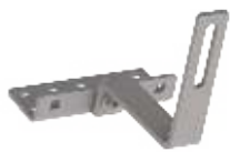
Universal Standard Hook +2, 5.5" Base" Material: aluminum Finish: mill Hardware: stainless steel
