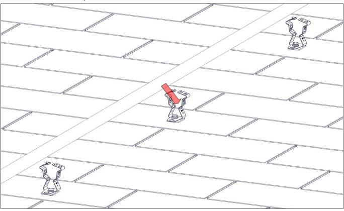
Secure conduit by pressing securement tabs closed to locking position for the appropriate conduit size.
