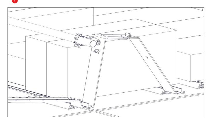
Secure conduit by pressing securement tabs closed to locking position for the appropriate conduit size. First securement tab hole will fit 1" conduit, and second hole will fit 3/4".
