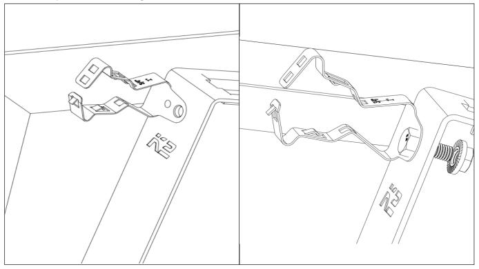
Hold Conduit Clamp in desired orientation while tightening the bolt and nut. Torque to (XX, I'm not sure what we are saying for torque value here, I'll try to find out if anyone has tested this.) Continue placing clamps along row of chassis, refer to local AHJ for maximum span between supports.
