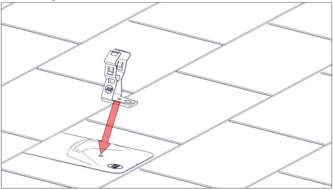
Using a 5/16" nut driver, fasten the provided wood screw through conduit clamp and flashing into roof decking, securing the clamp in desired orientation. To ensure the screw is properly fastened, drive the screw until sealing washer begins to spread. Do not overtorque or undertorque. See F1 below.
