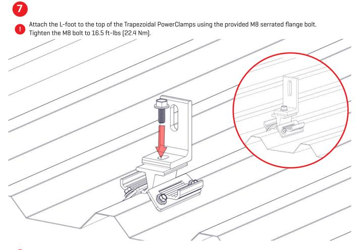
Repeat step 7 until you have all your L-feet secured and aligned straight on the Trapezoidal PowerClamps.
