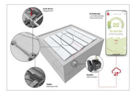
Structure and components of the K2 Buddy: Weighing unit, TopBox for data collection, BaseBox for data transmission and app for live data display (Image source: K2 Systems).
