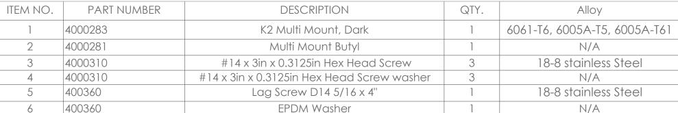
MULTI MOUNT FOR TILE ROOF MOUNTING (IN RAFTER)
