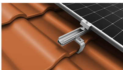
Less is often more: The bracket of the K2 SingleHook 3S Light is just 6 mm thick, so that it can be carried through with concrete roof tiles with less effort.
